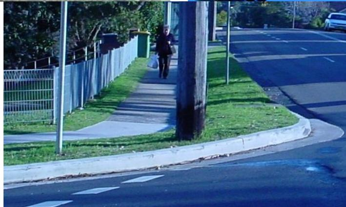
Basically the area between your front kerb and boundary is council owned and most councils require that the drainage from a property be conveyed across this area via gravity means. So as you can see from the photos for a pipeline to travel across this area with a fall to the street, it would need to connect to a council pipeline in the street as the kerb is too high.
